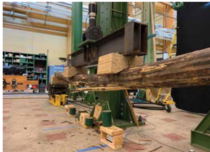
Figure 4. Red Pine ASTM D198 Flexural Testing at the USDA Forest Products Laboratory, Madison, WI.
