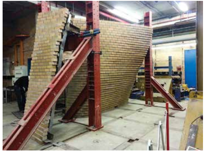
Figure 10. Full-size mockup panels before load testing.
