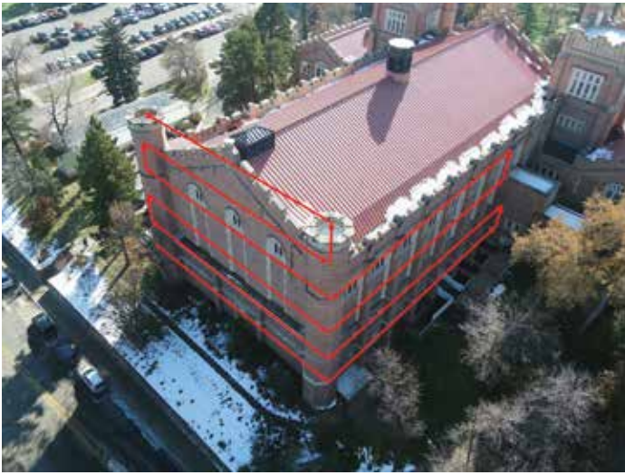
Figure 4. Preprogrammed flight path for façade mapping.
