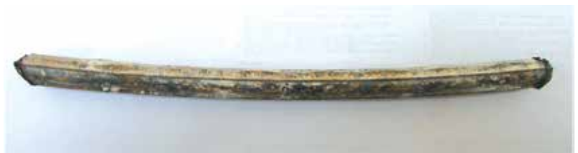
Figure 16. Feasibility analysis was based on top and bottom concentric reinforcing hoops with a 27 ksi yield strength resulting from a laboratory test of this sample.
