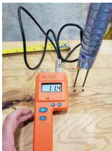
Figure 1. Initial moisture content with standard prong.
