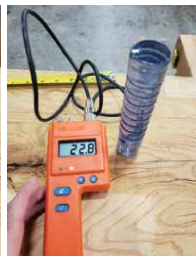
Figure 2. Initial moisture content 3 inches below surface.
