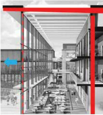
Schematic section at Commons showing the framing geometry of the column (right), glass wall (left) and the roof cantilevers (top).
