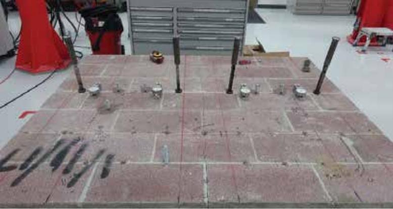
Figure 2. Generating a crack in masonry members for anchorage testing.
