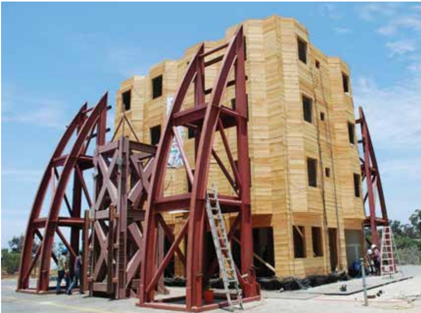
Figure 7. Shake table testing at UC San Diego, as part of the NEES-Soft program.
