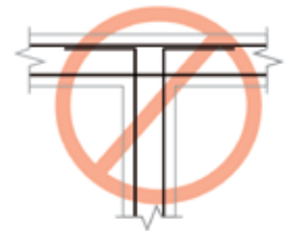
Figure 9. Wall intersection detail that should be avoided – double layers of transverse reinforcement.
