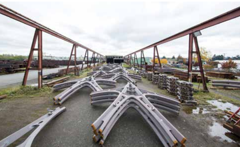
Figure 4. Steel fabrication of the Catalan pieces. Courtesy of NBBJ/Sean Airhart.
