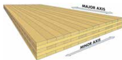
CLT panels are available up to 10 feet wide and over 60 feet long. Courtesy of WoodWorks.
