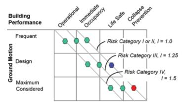
Figure 1. Expected seismic performance of buildings assigned to different seismic design categories. Courtesy of FEMA P-1050-1.
