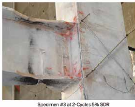
Figure 6. SMF Specimen #3 test results (UCSD).
