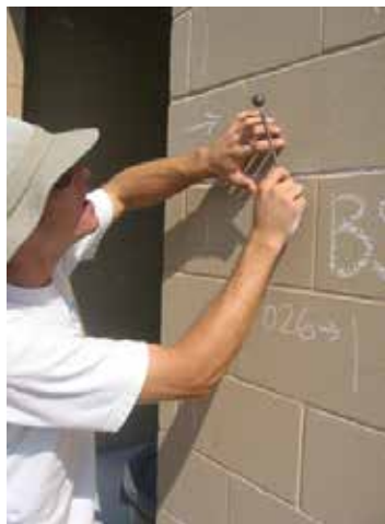
Figure 2. Sounding hammer used to locate hollow and grouted cells in concrete masonry construction.
