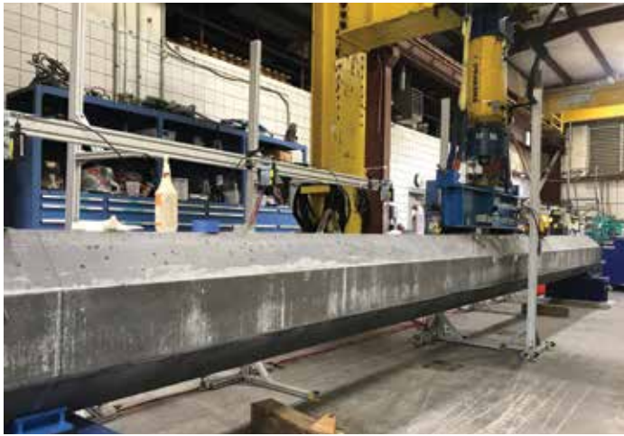
Figure 4. UHPC pile being tested at the Structures Laboratory of Florida DOT.
