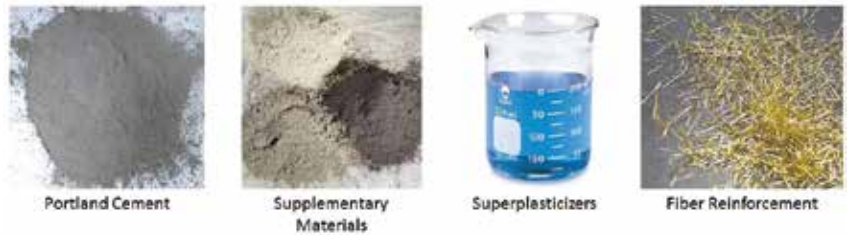
Figure 2. Components of Ultra-High-Performance Concrete (UHPC).
