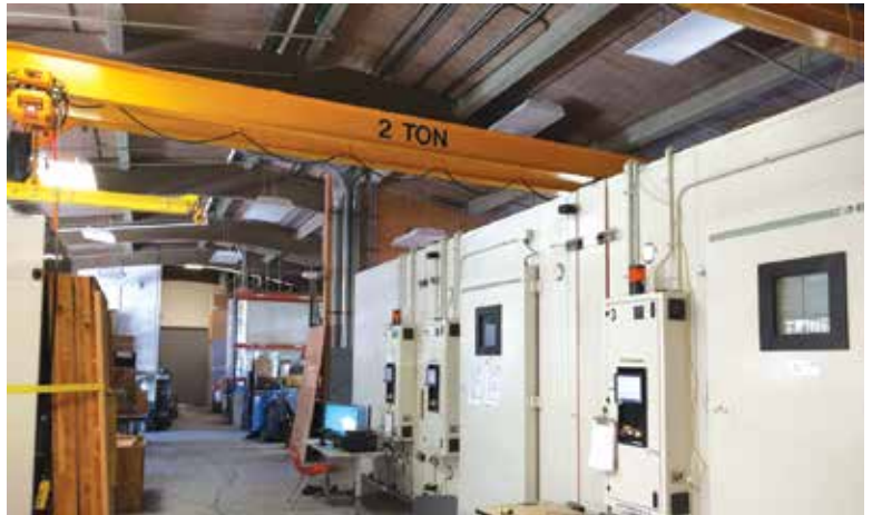
The MCMEC (Multi-Chamber Modular Environmental Conditioning System), where CLT samples will be exposed to varying environmental conditions during the first stages of the new USDA and TDI funded research.
