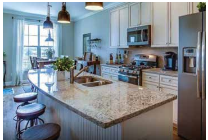
Figure 4. Kitchen island oriented parallel to the floor framing. For this case, almost the entire weight of the island would be supported by two framing members at 24 inches on-center.
