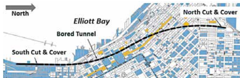
Figure 1. SR 99 Bored Tunnel and Approaches.
