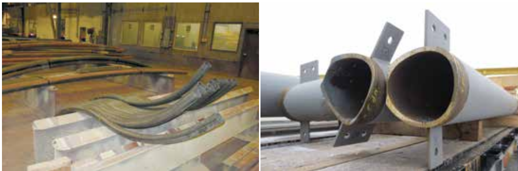
Figure 2. HSS prior to final cutting (left) and birds-mouth cuts (right).
