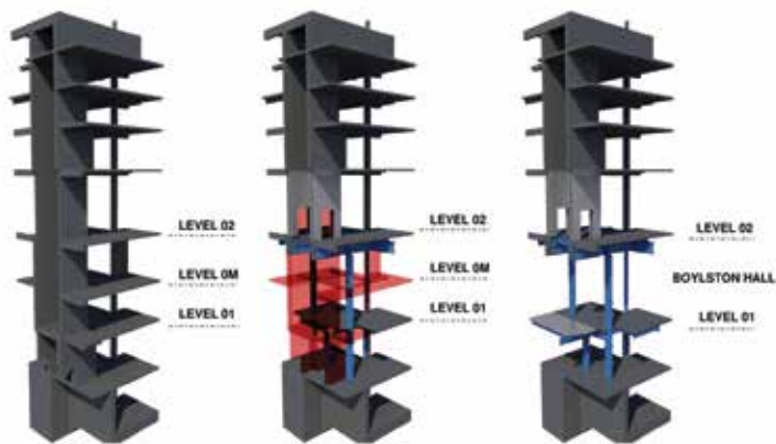
Left: 1972 construction. Center: steel framing installed. Removed structure highlighted in red. Right: Final condition.
