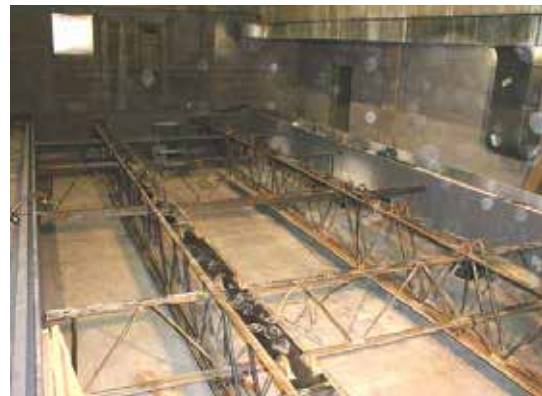
Figure 1a. Structural floor assembly for ASTM E119 test.
