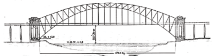
SPANDREL BRACED ARCH DESIGN (1905)
