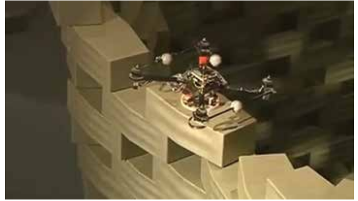
Figure 4. Drones are building a block structure.
