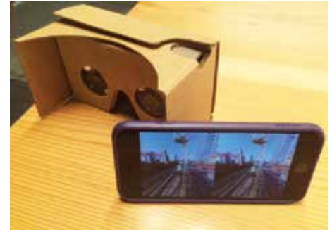
With the use of an inexpensive cardboard headset kit and a smartphone, viewers can experience VR at their fingertips. Featured here is an as-built pre-pour panoramic view with comments.
