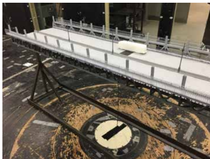
Figure 9. Wind on vehicle test. Courtesy of Boundary Layer Wind Tunnel Laboratory.
