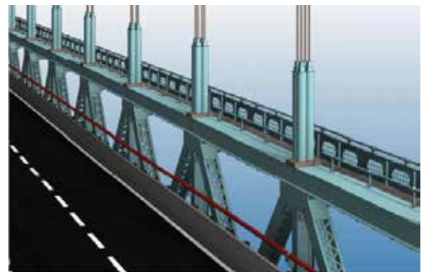
Figure 4. Perforations in sidewalk fascia girder.
