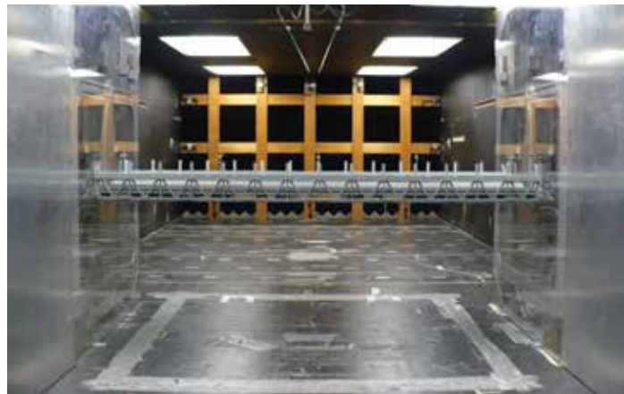
Figure 7. Section model test with turbulence. Courtesy of Boundary Layer Wind Tunnel Laboratory.
