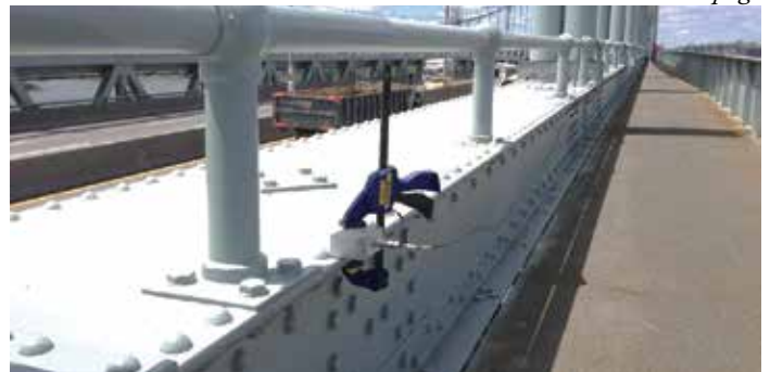
Figure 8 and 9. Tri-axial accelerometers attached to the bridge. Courtesy of Thornton Tomasetti Weidlinger.
