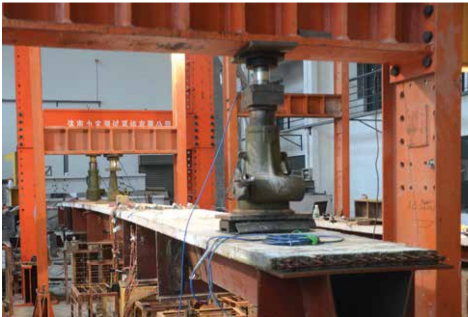
Figure 3. Set-up of the static load test.
