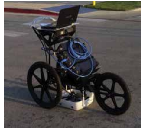
Figure 4. Bridge Inspection Unit with single antennae. Courtesy of GSSI and Echem Consultants LLC.
