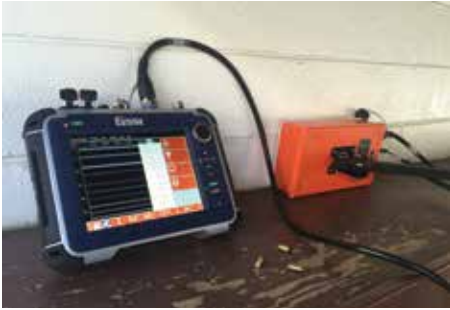
Figure 3. SIR4000 GSSI GPR equipment – 2016. Courtesy of GSSI and Echem Consultants LLC.
