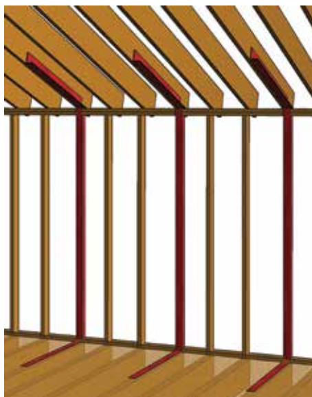
Figure 3. Schematic view of vehicle retention posts within the rear wall of the garage.
