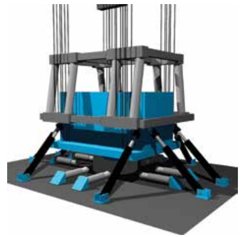
Design of TMD systems using ITT Enidine fluid viscous damper technology increases occupant comfort, reduces life cycle costs, and increases safety.
