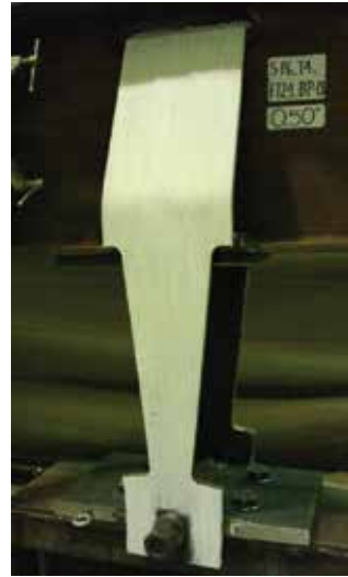
Figure 4. Successful bent welded fuse connector plates on either side of beam to masonry panel connection.
