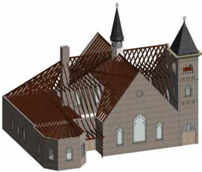
Figure 2. Ceiling and roof framing from the church in Case Study one.
