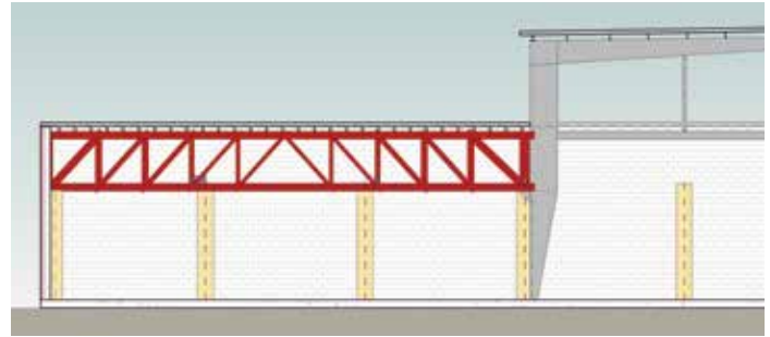
Figure 3. Section of the pre-engineered metal bay and wood truss bay in the building from Case Study two.
