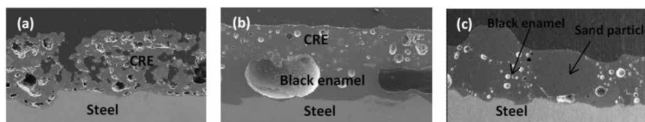
Figure 2. Microstructure of (a) chemical reactive enamel (CRE), (b) double enamel, and (c) sand particle modified enamel.
