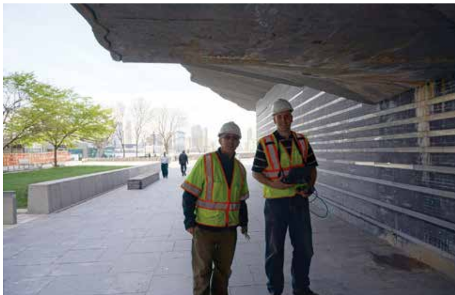
Figure 2. Team getting ready to perform LPR test at location in New York City, May 2015.
