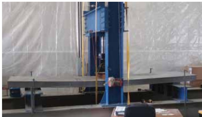
Figure 4. CA performs bending test on FRP deck panel to design loads and safety factors.
