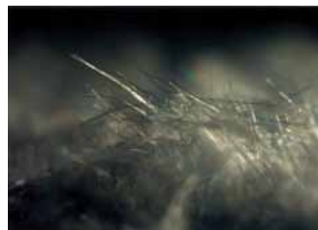
When reacting with water and cement, an ICW creates millions of needle-like crystals that block the ingress of water. Courtesy of Kryton International Inc.
