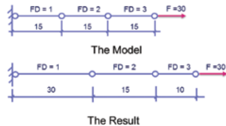
Figure 13. Force Density form-finding.
