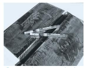
Temperature-indicating crayons such as these Tempilstiks<sup>TM</sup> are used to measure preheat and interpass temperatures.
