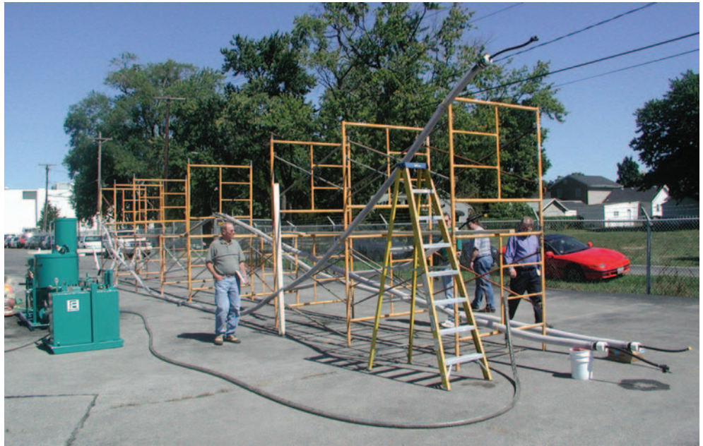
Setup for the Full Scale Grouting Mock-Up for the Maumee River Bridge.
