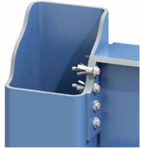
Figure 1. A 3D model illustrates a structural connection and shows how the bolt expands inside the HSS section.
