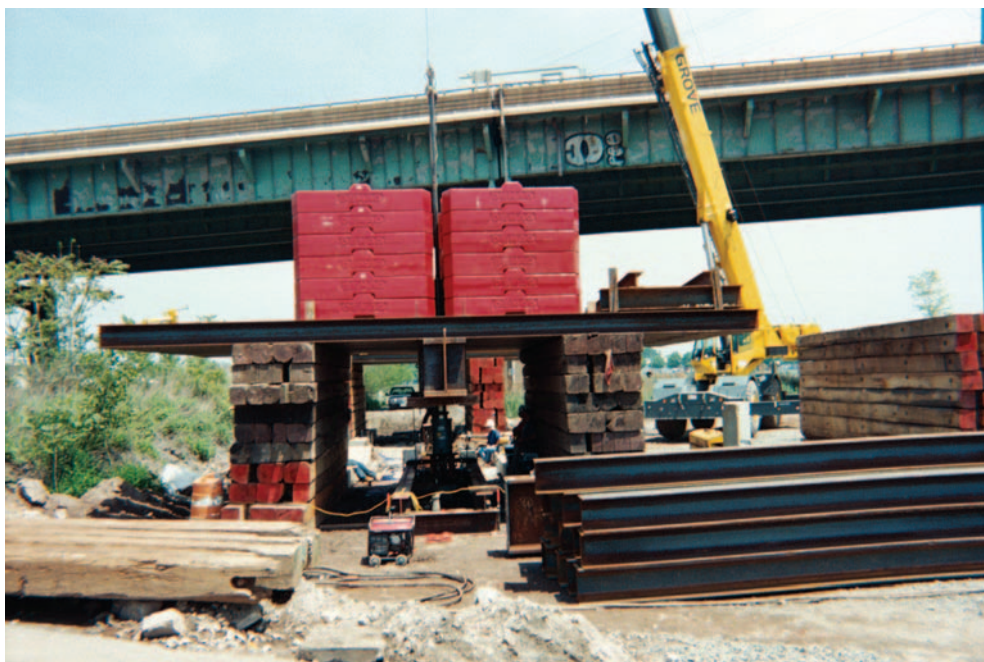
Figure 1: Static Load Test with Dead Weight Reaction, New Haven, CT
