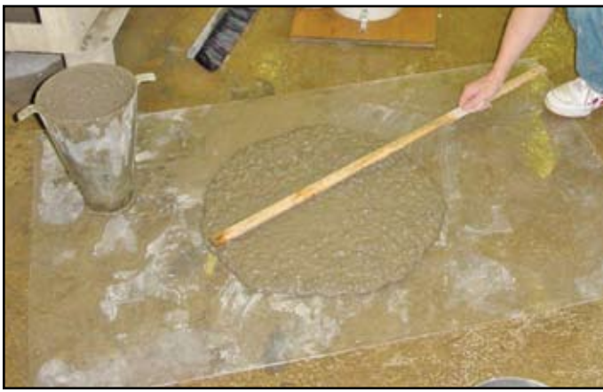
Figure 2: The slump flow test (ASTM C1611) demonstrates the high flowability of SCC
