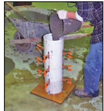
Figure 3: The column segregation test (ASTM C1610) can be used for detecting static segregation in SCC
