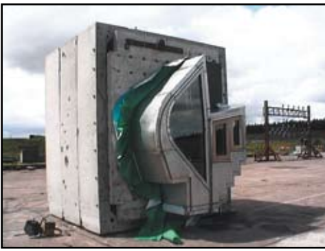
Figure 4: Arrangement for Full-scale Testing of the Blast Resistance of Exterior Windows in the Scottish Parliament Building. ©Arup
