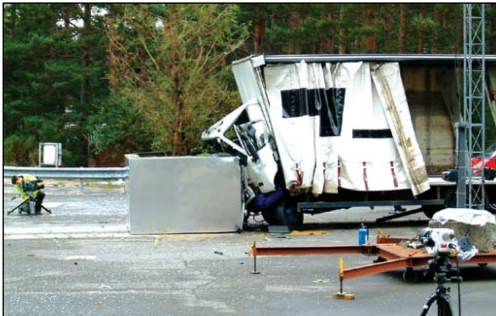
Figure 3: Full-scale Test of Vehicle Barrier System. ©Arup/David Hadden
