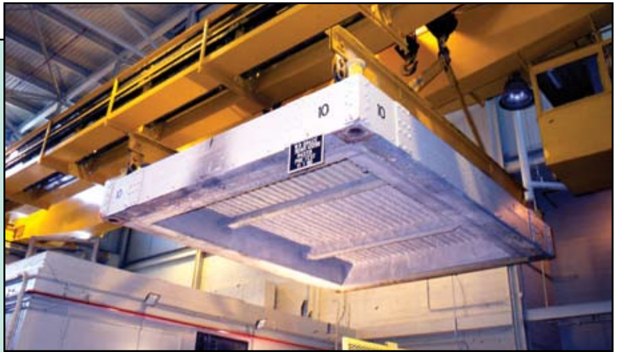
UL: View of a floor assembly being lowered onto the UL Test Chamber.
