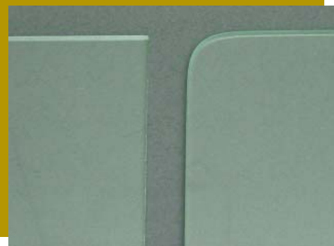
Figure 4: Rounded Corner Glass Panel Can Provide Greater Cracking Drift Capacity
