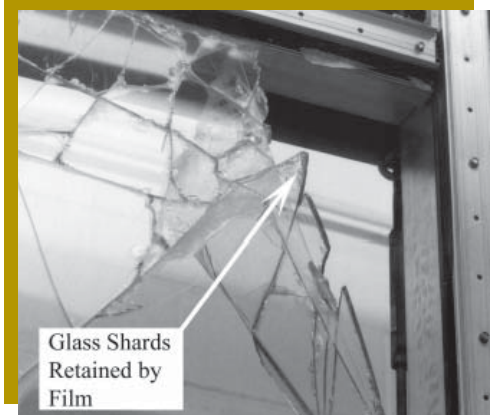
Figure 3: Application of PET Film and How Glass Shards Are Retained by PET Film
