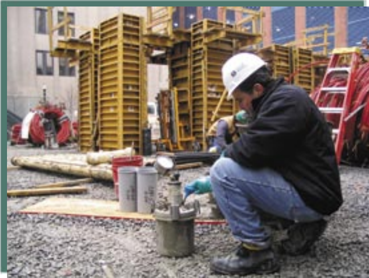
Field testing of concrete is a key element of quality control. Excessive testing, however, does not add to quality and can be counterproductive
