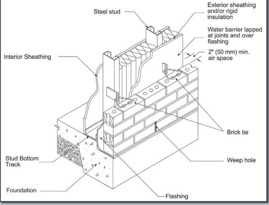
Figure 1: Steel Stud Brick Veneer Wall System
