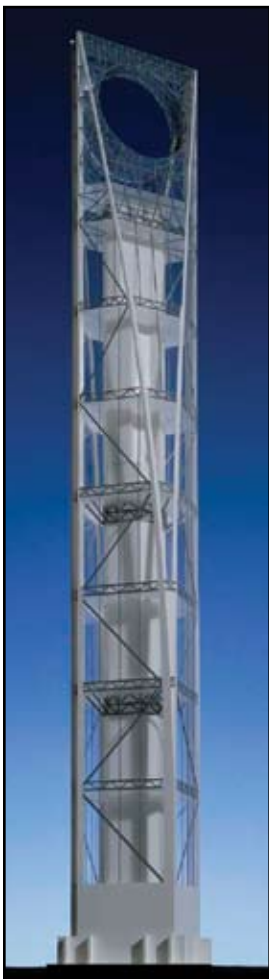
Figure 2: Structural Model – Omitting Intermediate Floors. Courtesy of Jock Pottle.
