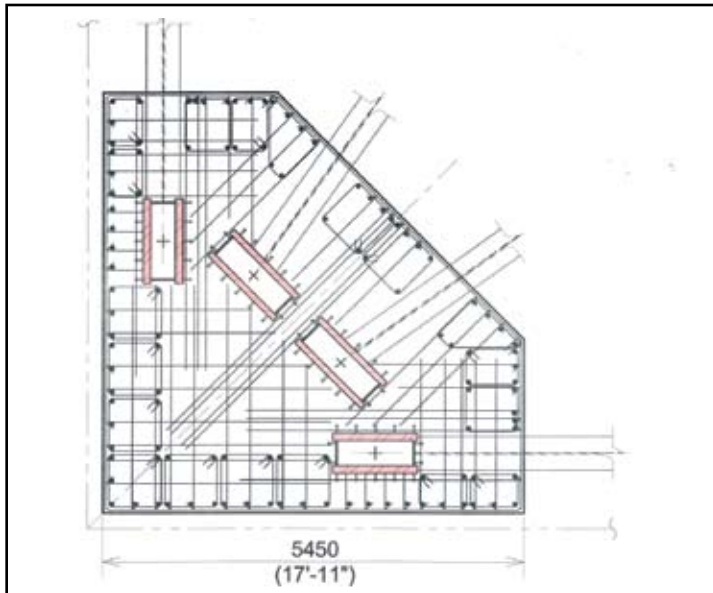
Figure 6: Mega Column at Base.
