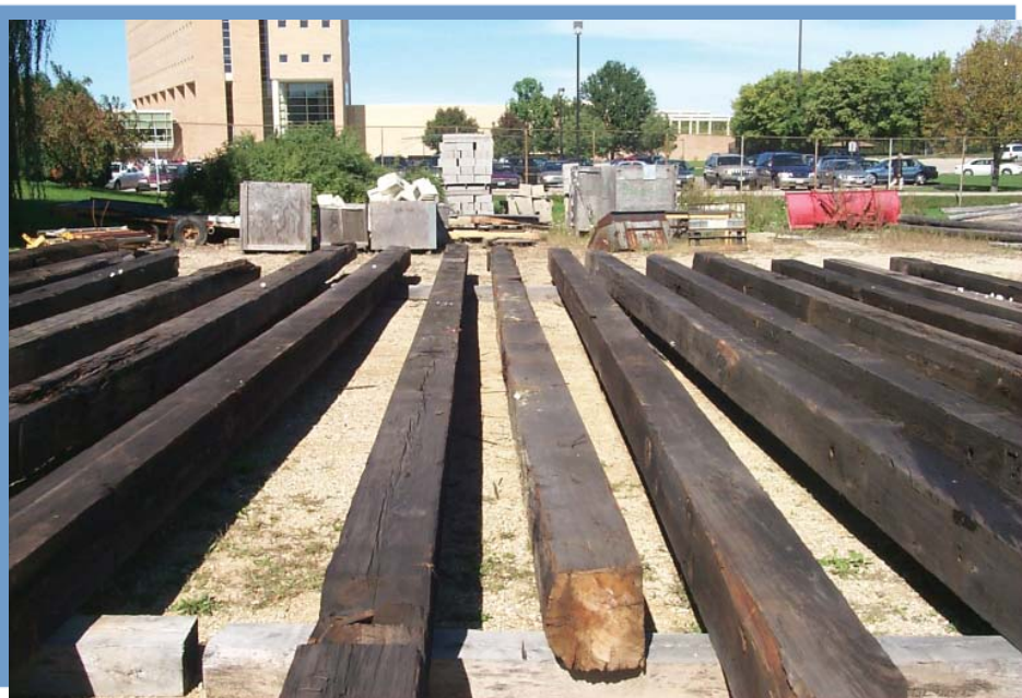
Figure 1: Fifteen 12-by 12-inch white pine timbers removed from the Quincy Mine Blacksmith Shop
