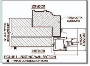
8-inch wall for wind resistance. In most areas, the strength of the wall was maintained by the use of cold form stud construction let in to the masonry substrate, particularly where terra cotta surrounds were removed. According to Massachusetts Building Code, 780 CMR, Chapter 34, as a historical structure, as well
